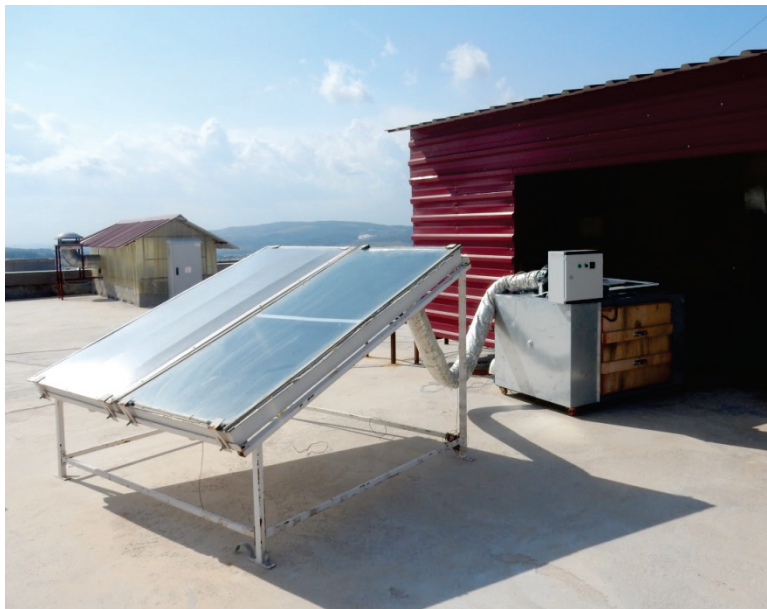
Figure 1 Schematic illustration (a) and the image (b) of the solar-assisted drying system
